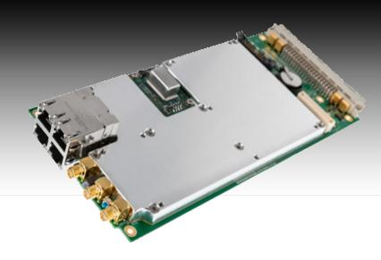
The PT3160 ATSC OEM ProTelevision Technologies Software defined modulator provides maximum integration flexibility for transmitter manufacturers.
